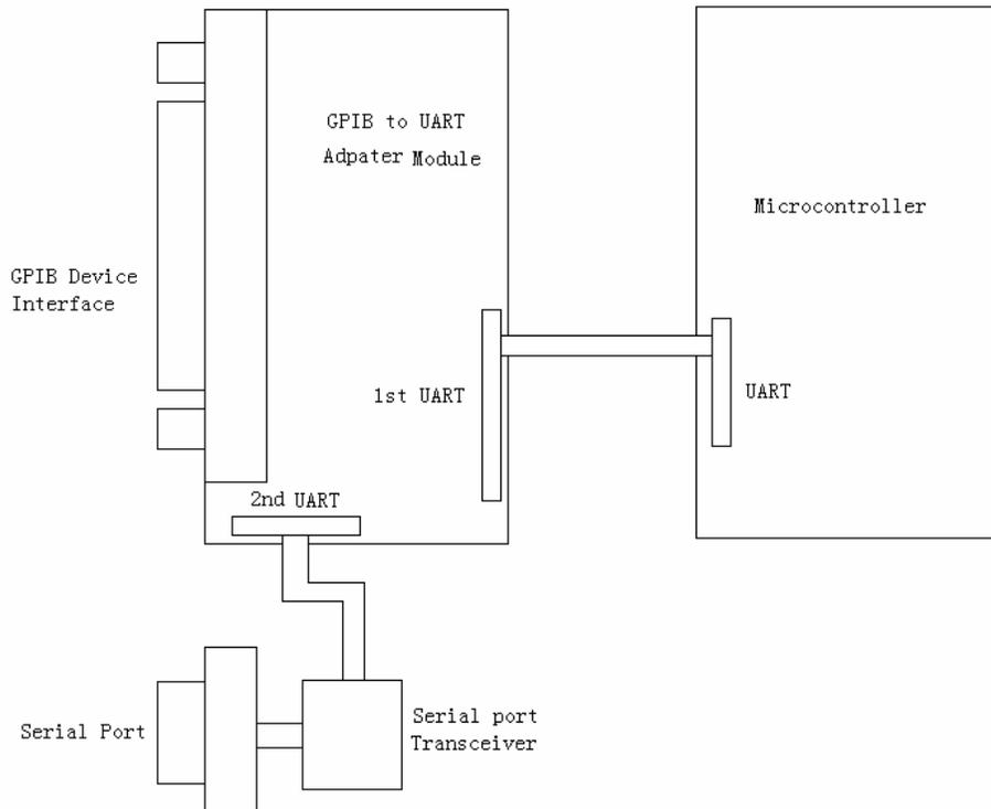
Fig. 4 GPIB Device interface to UART Adapter with UART serial port
